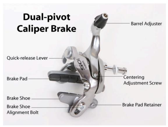
"Dual-pivot" brakes are a high-end variety of side-pull, uses hex nuts, better materials
