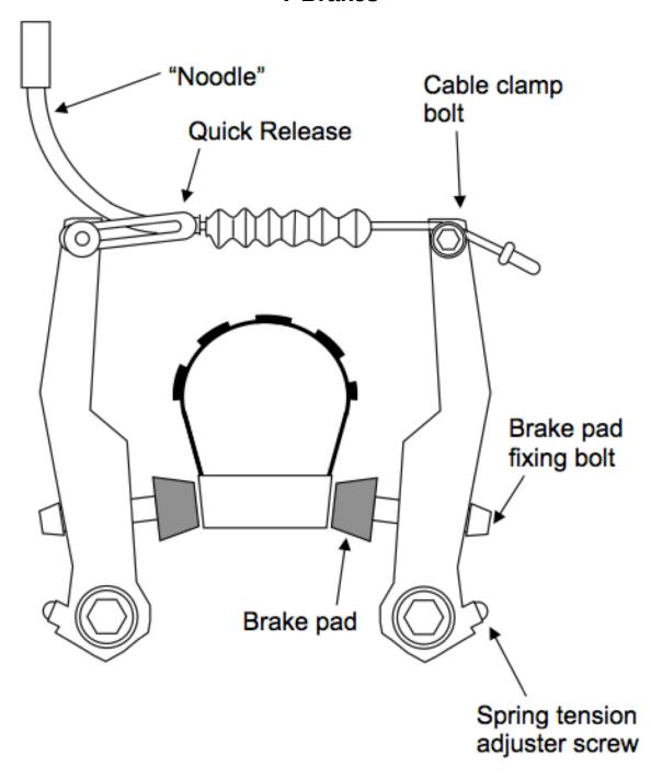
Tightening a spring tension screw increases tension, moves pad closer to rim
