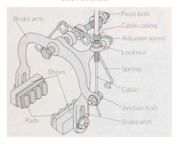
This diagram is for a side-pull brake on a low-end bike
