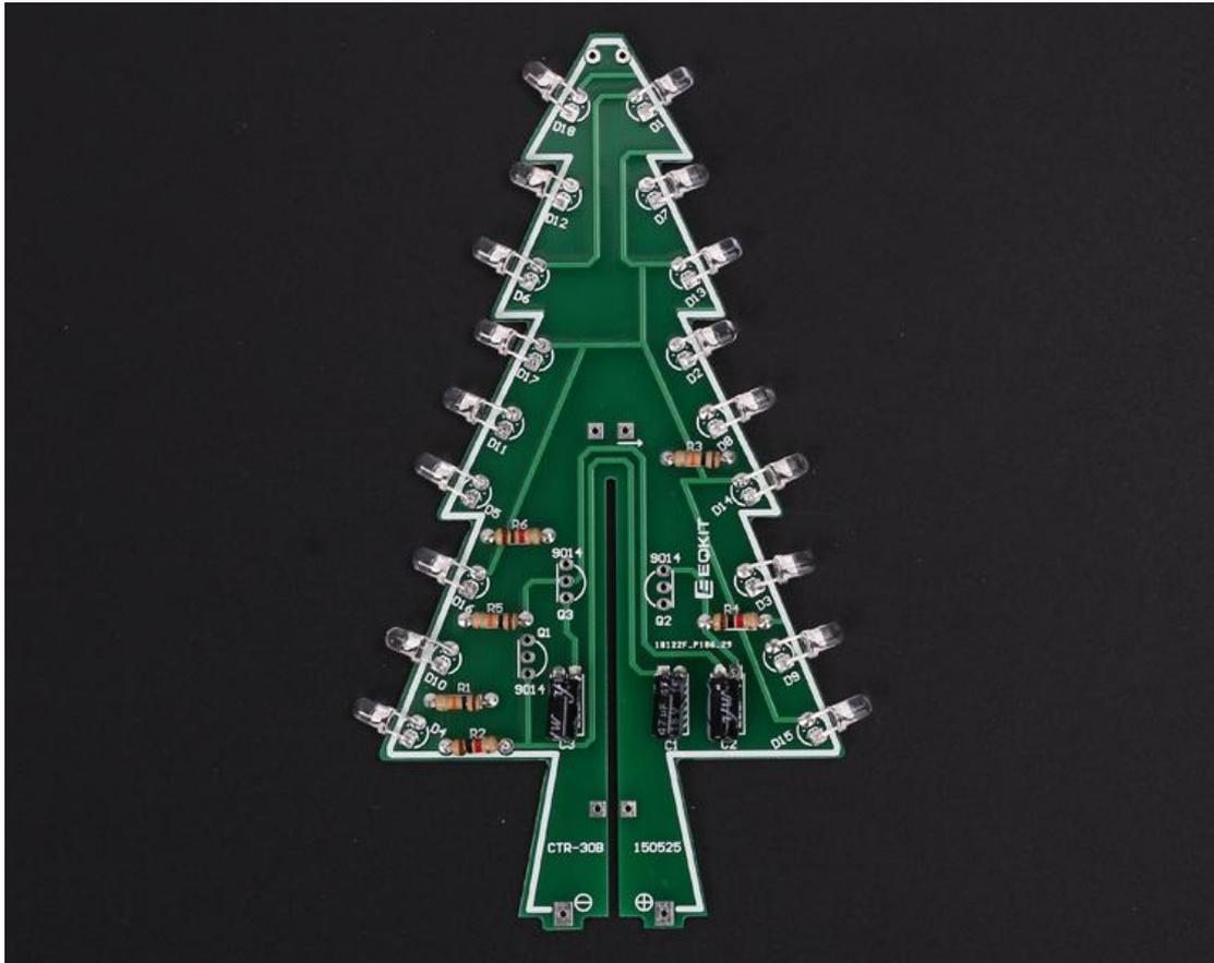
Step 11: Install 3pcs TO-92 S9014 Transistor
