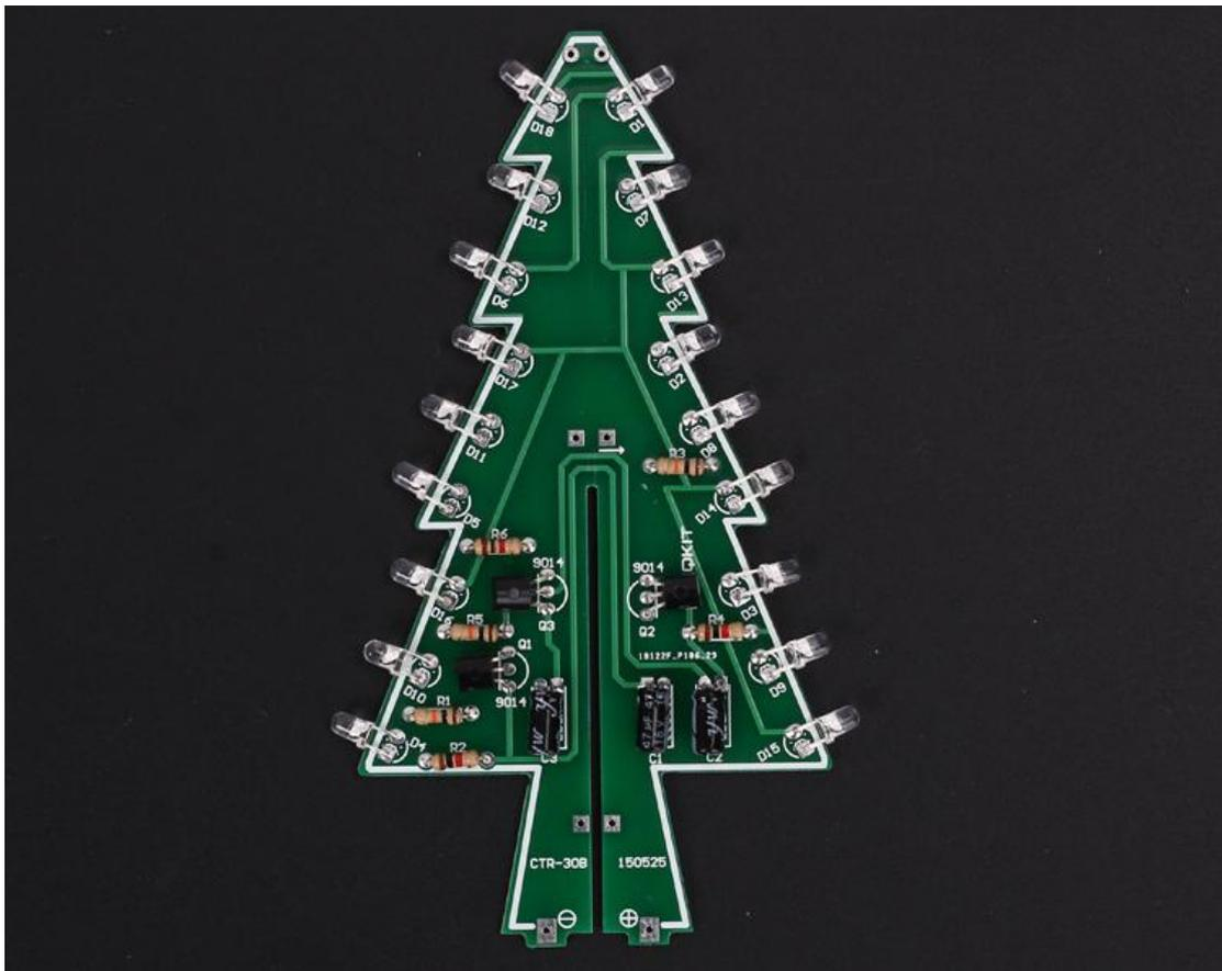
Step 12: Connect 5V to CTR-30A and CTR-30B. Preliminary welding success if LEDs are blinking automatically
