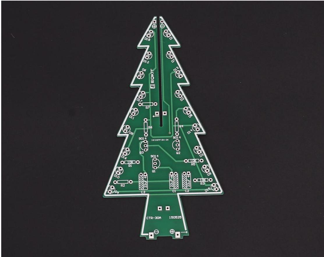
Step 1: Install 3pcs 1K Metal Film Resistor on R2,R4,R6
