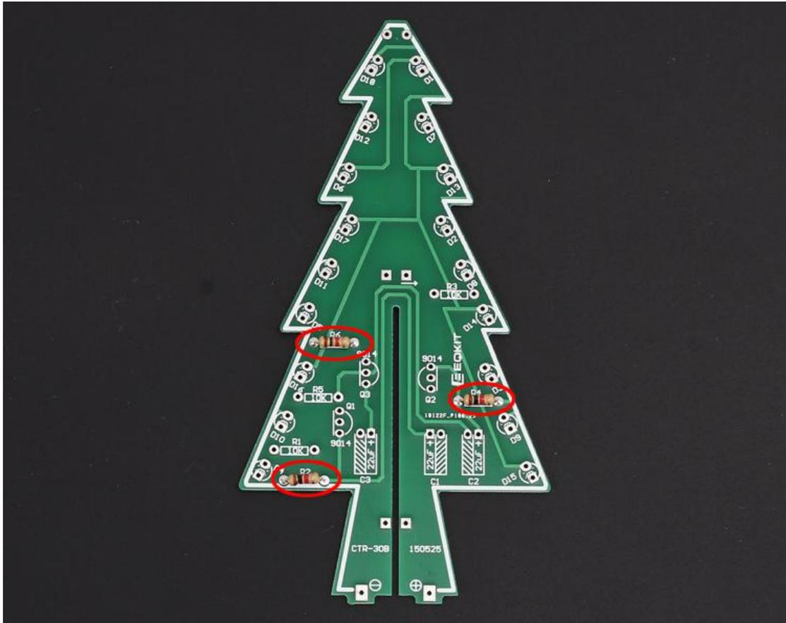
Step 8: Install 3pcs 10K Metal Film Resistor on R1,R3,R5
