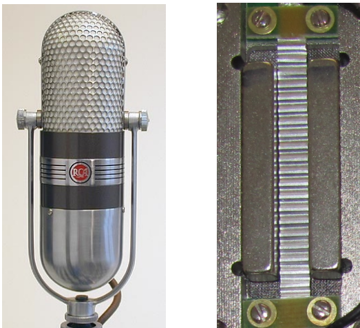
Fig. 1: Classic RCA 77D Microphone (left) [21], and corrugated ribbon from a Nady RSM-4 ribbon microphone (right). The corrugations stiffen the ribbon against off-axis motion.
