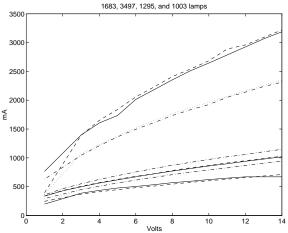
Here is another odd one. The lowest trace on this chart represents the 1683 lamps, the next one up the 1003 and 93 lamps, and the top two groupings are the 3498 and (topmost) 1295 lamps. The first set of measurements I did of the 1683 lamps showed a severe nonlinearity at low voltages but this does not seem to be repeatable at all.
