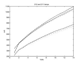
This figure shows measurements of various 211 and 212 lamps, again from different manufacturers. Some of these lamps appear to show a knee on the lowest measurement. It is, however, a very slight one and may well be a measurement error. Note that the lower trace here represents the 212 lamps, while the upper trace represents the 211 lamps.
