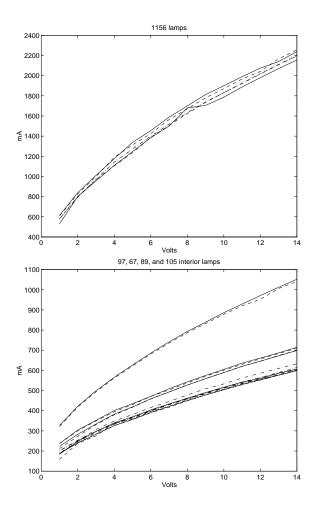
The figures above show the actual measurement of various lamps from different manufacturers and of different types. As you can see, the curves are fairly smooth with no real knee, and the limiting effect begins well below the point at which a glow is visible by the naked eye.
