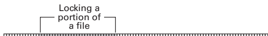
Figure 1.18 A lock can be acquired over a portion of a file. This portion must be contiguous.
